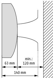
**Montage des KNX 4 DC Motor Controller WM**
